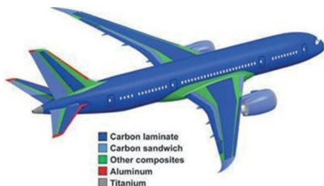
Figure 5. Composition of composites in B787 Dreamliner.
